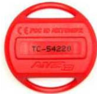
This illustration shows the correct orientation for the transponder in the canister. The number should face forward and the transponder should be vertical.
