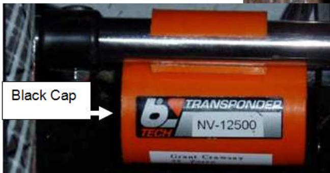
Now put the cap back on so the logo "b" faces the right way. Then if you have any doubt about how to put the canister on the kart, just check that the "b" logo is the right way up and the label faces forward. Re-locate the transponder canister on your kart as shown above.
