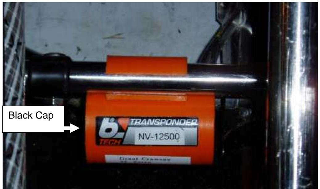
Note that the transponder is positioned on the small front bar on the right hand side of the kart, just below where your calf muscle would be if you were sitting in the kart. This position also makes it hard to kick it off by mistake with your foot because the closed part of the mount faces rearwards. Also it will not rub your leg. It may swing backwards and forwards but this is OK.
